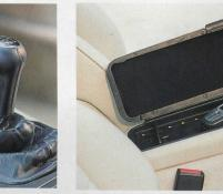
th use Central armrest has a lifting lid with a rather crude plastic hinge that eventually breaks. Inside would originally k has have been plastic cassette-tape holders — which often break, too. In these days of CDs it makes sense to remove these troublesome items and use the space for useful oddments storage, as above
