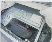
In the rear compartment lift the carpet (check that it's dry) and make sure that the space-saver spare wheel and compressor are present. Original toolkit is not only a nice feature, but also contains a special spanner for the deepset spark plugs. Make sure both the jack and its handle are present – and work!
