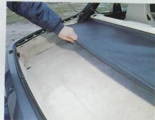
Check that the luggage-compartment blind is intact and pulls neatly across without sagging, and rolls back under its own steam when required. This item often deteriorates after long exposure to sunlight. But replacement blinds are available, and relatively simple to fit
