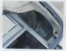
Check that the deep wells on each side of the luggage compartment (the battery is in the left-hand one in the S2) are nice and dry. Drain tubes from the sunroof are routed through them, and if these become detached and/or blocked rainwater can end up in the wells, especially if the drain holes are blocked
