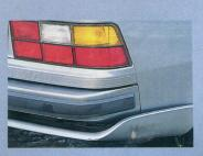
Rear under-spoiler (see detail, above) is a distinctive feature of the S2 (and later Turbos). It's vulnerable to damage, so check for cracks and repairs Door handles can become stiff, but they're easy enough to dismantle and squirt with penetrating oil. Open the doors and check the steel check-straps aren't loose. They should be welded to the 'A' pillar but often become detached, and it's not a simple job to repair them Door mirrors are susceptible to scrapes and stone-chips.
