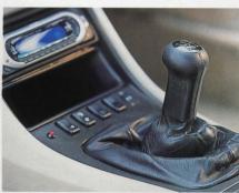
Gear-lever gaiter tends to wear with use (although the one in this car is surprisingly good). If a replacement has been fitted make sure that the work has been done neatly. Annoying buzzing noise from gear lever at high speed can often be cured simply by removing the covering trim and replacing it again
