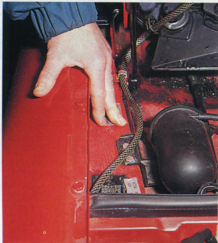
Distortion here is a sure sign the car has suffered a frontal impact
