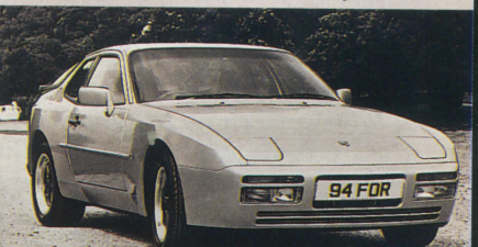
Early 944 Turbo has 220bhp, later cars 250bhp
