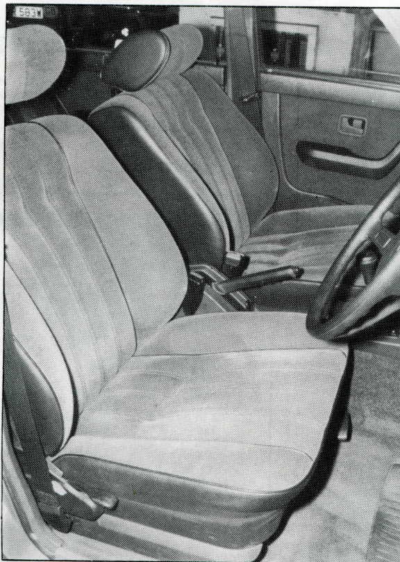
Although somewhat on the firm side, the seats are large and comfortable. In addition to the usual backrest adjustment, the driver's seat cushion is adjustable for height and angle. The steering wheel is reach-adjustable
