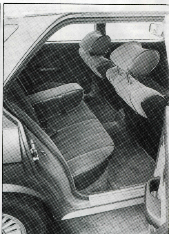
Although somewhat on the firm side, the seats are large and comfortable. In addition to the usual backrest adjustment, the driver's seat cushion is adjustable for height and angle. The steering wheel is reach-adjustable
